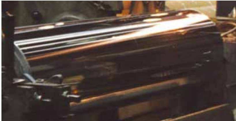
Wear-resistant tungsten carbide coatings last three to five times longer than welded repairs.
