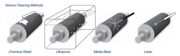
This Hard Facts looks at some of the cleaning systems that are used to restore the ink-carrying capacity of a laser engraved ceramic anilox roll, by removing deposits that are clogging/plugging the roll's cell structure.
