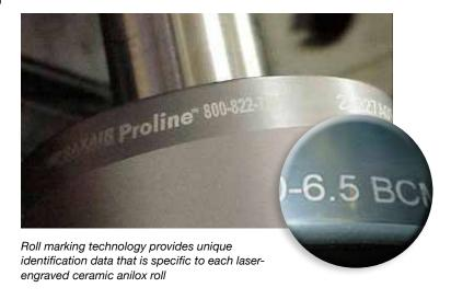
In addition, when you need to have rollers re-engraved or want to specify the requirements for a new order, having an identification band on your roll provides you with easily obtained and detailed information, which eliminates the time required to research data for a new order.
