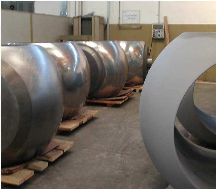
Praxair can coat ball valves up to 56" in diameter
