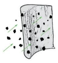
Over time, ash and other particulates erode fan blades and hubs, lowering efficiency and shortening their working life.
