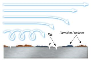
In addition to erosion damage, particles in the air can condense and dry on blade surfaces, causing pits, cracks, and other damage.
