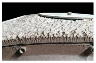
Corrosion has left this hub pitted and rough, adding to fan drag and wear. Praxair coating solutions protect hubs against corrosion, for better wear life and fan performance.
