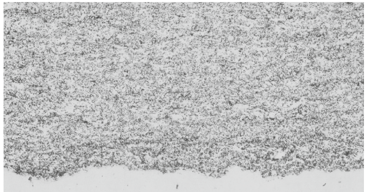
Typical 5220 gun Tungsten Carbide - 17% Cobalt Coating Microstructure
