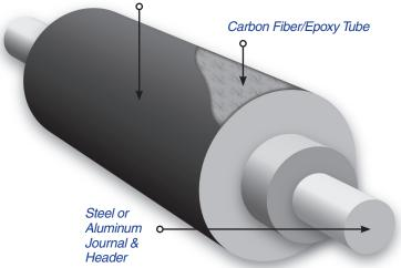
Praxair Surface Technologies has developed the technology that next allows the application of chromium oxide ceramic wear-resistant coating to the composite roll assembly. This is the the anilox roll and the plate over the entire length of the roll - a characteristic that maintains a more consistent print density across the web.
