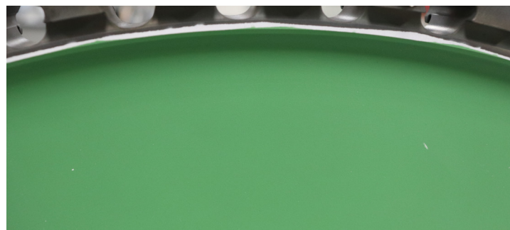
After quench adhesion test at 1400°F (760°C)
