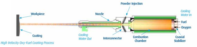
The most frequently used coating compositions are carbide-based cermets, metals and alloys, and some oxides with sufficiently low melting points.
