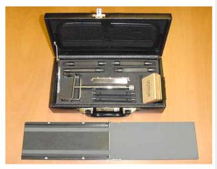
mechanism. The engraved anilox roll is next inserted in this mechanism, along with the doctor blade. The doctor blade pressure can being regulated by the screw in the handle of the device. Finally, the ink transfer plate is opened and placed on a flat level surface with the guide rails facing up.
