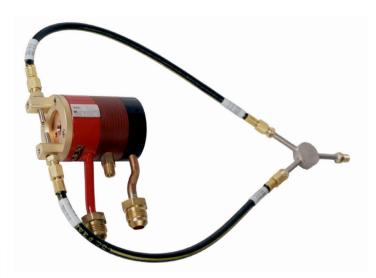
Dual port external powder injection with variable port angles is available as an option for both the Model SG-100 and SG-200 (above). These external ports can be used in place of, or in conjunction with, the internal ports.
