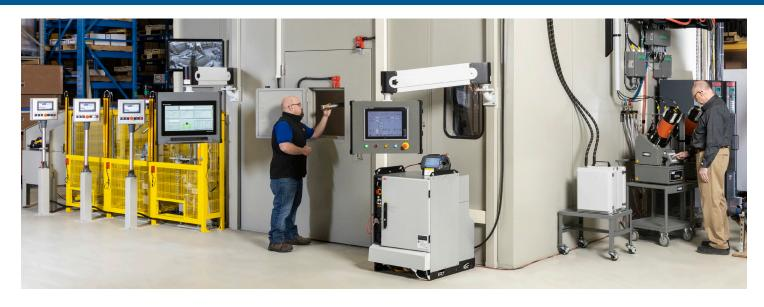
Our 7700-based plasma systems are designed for easy integration with the 7780 Universal Process Control Center (UPCC), a sophisticated multi-process thermal spray controller. 7780 UPCC technology allows a single workstation to control multiple thermal spray systems such as plasma, HE plasma, PlazJet, GF-HVOF, HP/HVOF, combustion powder and wire, and Arc Spray.
