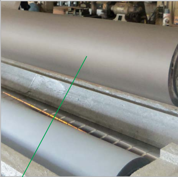
Before zinc submersion, this roll coated and sealed with the Praxair carbide coating/chrome-free sealer system has a uniform, chemically-bonded surface.
