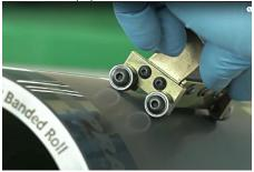
4. Electrostatic copy paper is then placed against the roll and rubbed over the ink area. When the paper is removed, the ink will have transferred to the paper in a pattern representing the inked surface area. Clean the roll.
