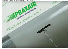
3. Once ink has been applied to the roll surface, the URMI tractor assembly, containing a clean-edged doctor blade, is used to evenly spread the ink.
