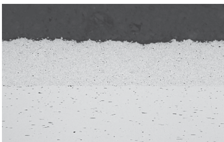
ExoGreen coating cross-section showing dense microstructure
