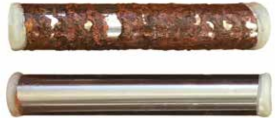
Hard chrome vs. ExoGreen salt fog test results after 1000 hours
