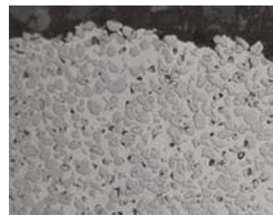
Figure 2. Tribomet T104CS coating microstructure
